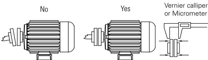
**NOTE:** The pulley should always be mounted firmly against the shaft shoulder and should be a firm fit onto the shaft. Impact force must not be used.
