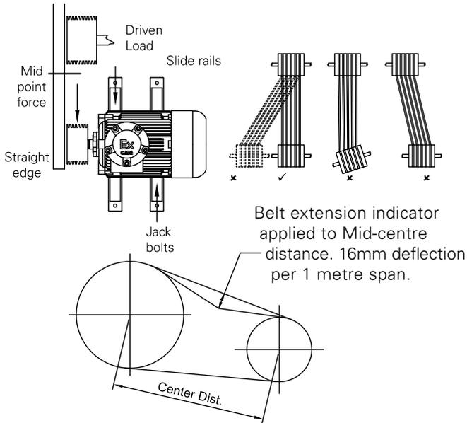
As a general rule the mid point of the applied force should be at the mid point of the shaft and it is good practice to mount the motor pulley with hub and locking screw at the shaft end.
