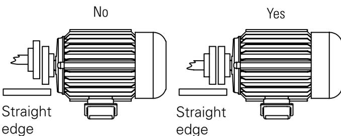
Excessive angular displacement must also be prevented. The recommended method to achieve correct angular alignment is shown below.
